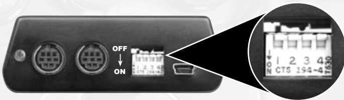
Fig. 1 Side view of interface with dip switches in correct position
